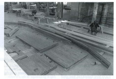
The main partition assembled, with kingposts and engine-room bulkhead.
