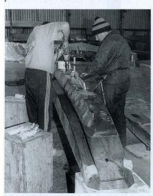
The stem bolted up and rabbets cut. Wayne Crow (with drill) and Nigel Armitage fitting the bobstay fitting.
